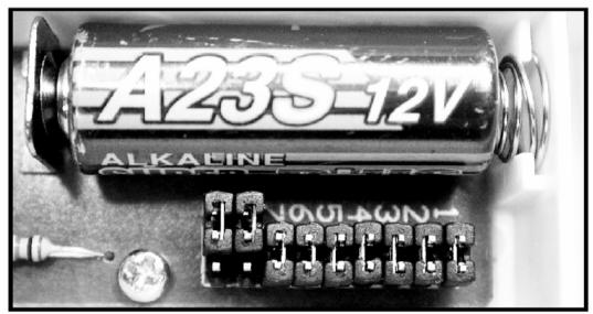
Parking the jumper on an open set of pins. The two jumpers on the left are in the parked position.
